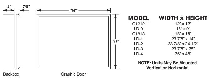
For Semi-flush mounting, add 3" to overall "W" and "H" dimensions.
