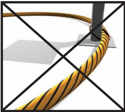
NOT RECOMMENDED Tye-Wrap to Floor Pedestal
